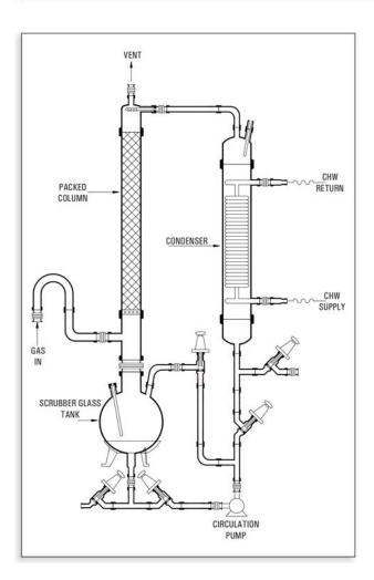
Goel offer Pilot Plant Gas Scrubber for various gases likes HCI, CI2, SO2, Br2, HBr, NOx etc or any other corrosive gases. These scrubbers use the media as water / Aq. NaOH / any other suitable solvent which can neutralise the exhaust gases. Our Pilot plant scrubber are ranging from 20L vessel capacity to 500L vessel capacity and scrubber diameter from 80DN to 300DN.
